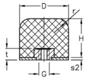
$$\begin{array}{lll} D & = 100 \\ d2 & = 4 \\ G & = M12 \\ H & = 80 \\ Load capacity F (kN) = 95.0 \\ Load capacity f (mm) = 44 \\ Load capacity W (J) & = 1120 \\ r & = 20.0 \\ \end{array}$$
